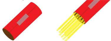
3) Finally, take the straw with the cone attached and put the straw through the toilet tissue tube. Take a little rubber/paper cement and glue the cone to the other end of the toilet tissue tube.
